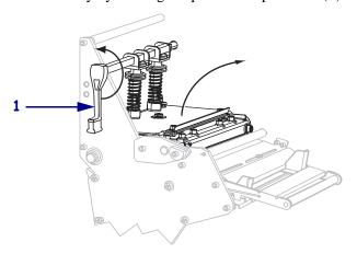
**4.** Loosen the thumb screw (not visible from this angle) that is located on the bottom of the outer media guide (1).
